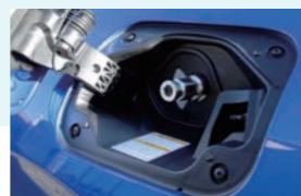
Hydrogen filling nozzle made with Aichi Steel stainless steel
