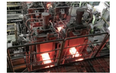
Small-section continuous casting machine for reducing CO 2 emissions (currently under development)
