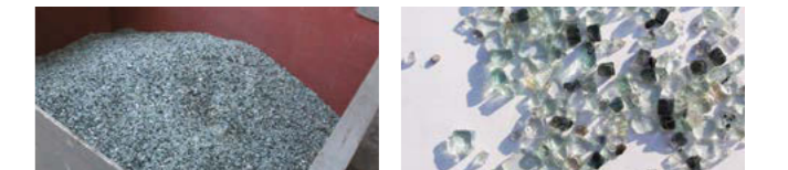
▲Waste glass from cars was previously difficult to recycle due to its specialty components and color
