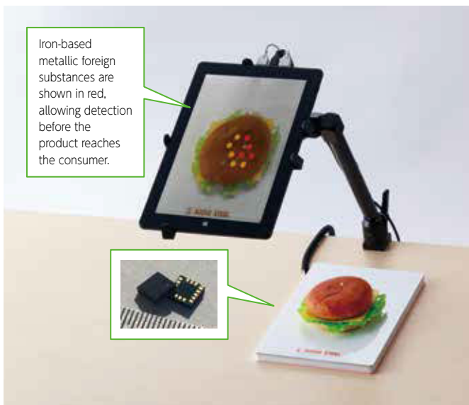
A mobile foreign substance detecting device using a tablet, and the MI Sensor
