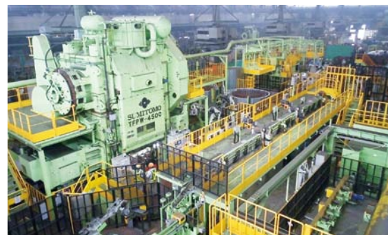
A 4,500-ton press at our forging plant
